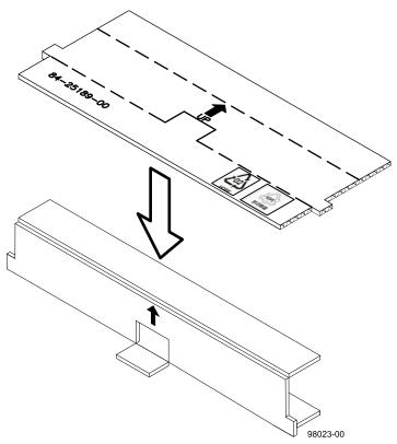
7. Remove the failed controller canister.
